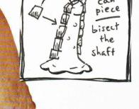
**4.** Mix the plaster with water. Cover the mold with the plaster. The aluminum squares are there so that the mold can come apart in halves, so do not cover those pieces completely. I would apply one thin coat and then another thin coat. The plaster needs to be able to dry and a thick coat won't dry even in a day or two's time. It is difficult to get a mold that will dry and not break apart, but you can do it. If the plaster needs to sit for a whole day, let it.
