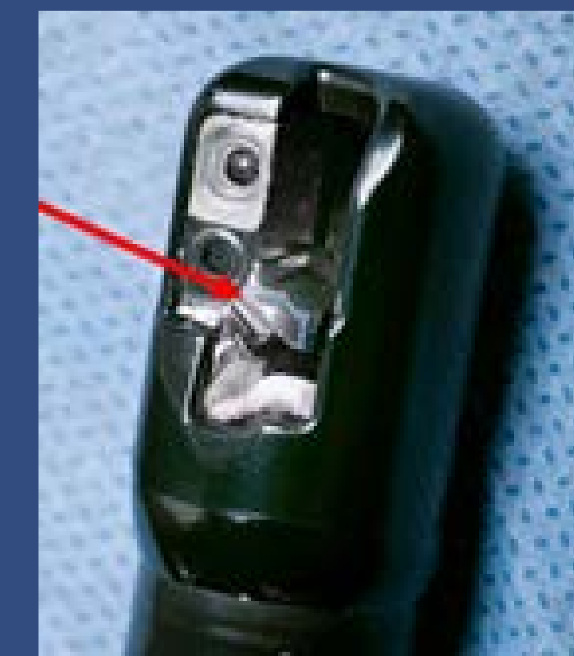
The elevator mechanism is challenging to clean
