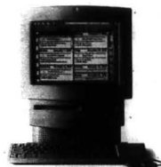
Macintosh LC 589 SBE, Internal AppleCD 300 CD-ROM Drive, Apple Keyboard II and mouse.
